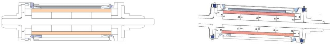
**Figure 7. The selected roller design with and without using small radial magnets at the collars of each roller end are seen with no basic difference in performance.**
