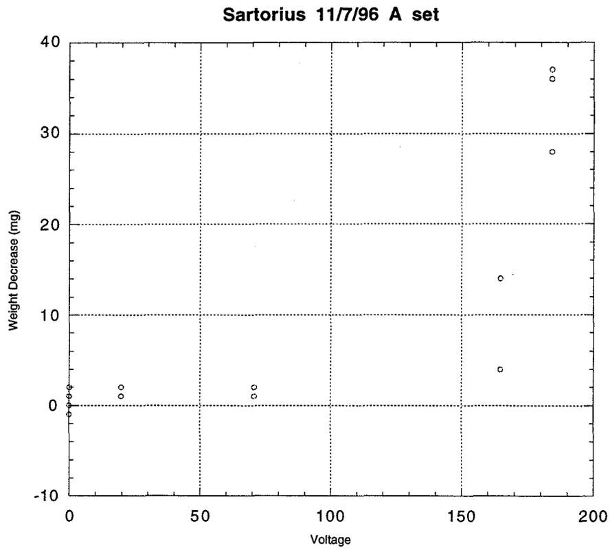
Figure 8. Weight loss of a rotorless gyroscope measured on a Sartorius scale as a function of applied voltage.
