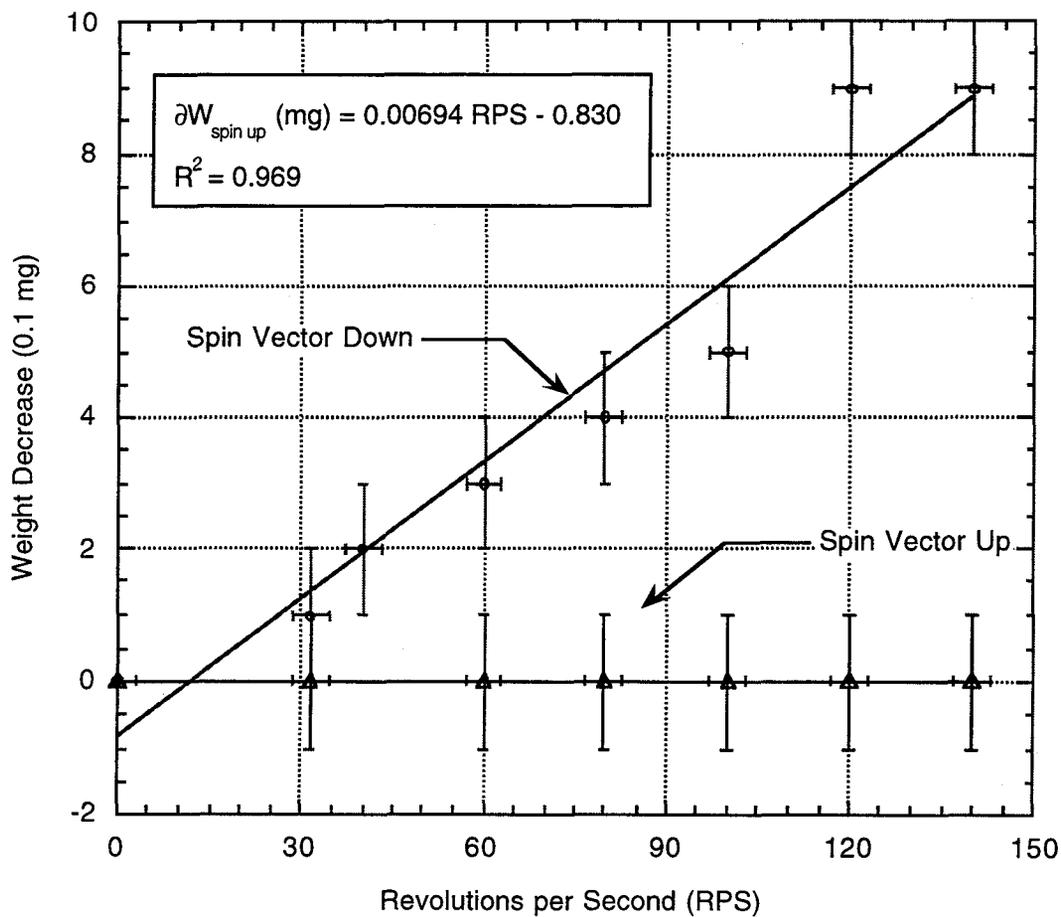
Figure 7. Weight loss measured on a Mettler scale as a function of rotation frequency of a gyroscope driven by three phase power. Sensitivity of the scale is 0.1mg.
